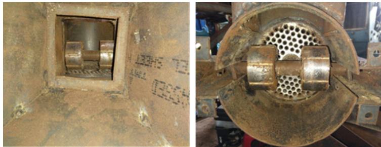
Figure 3. The horizontal roller and pellet mill flat die
