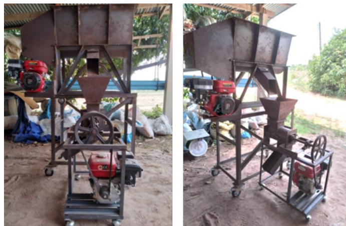
Figure 4. The mixer and pelletizer machine for organic fertilizer from cricket dung
